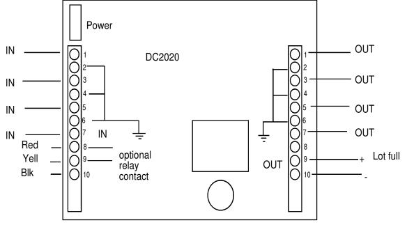
DC202 can directly interface to the Sysparc lot full sign. In this regards, the lot full sign will receive electrical supply (12VDC) directly from the DC2020.
